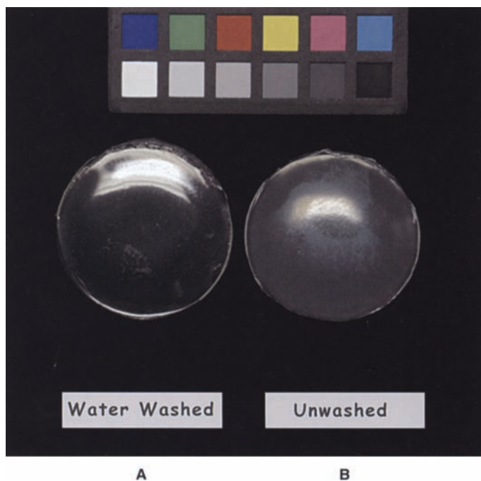
FIGURE 1 Surfactant exudates on pours of acrylic dispersion polymer (both pours are two weeks old): (A) soaked in water for 10 minutes, (B) untreated.
