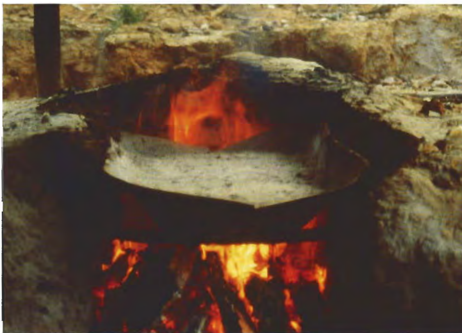
Figure 16. The heat treatment of amethyst to produce citrine at Marabá is simple but dramatic. The amethyst crystals are buried in sand in wheelbarrows and then heated over a wood fire.
