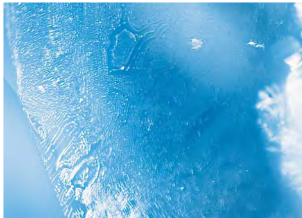
Figure 10. In a number of the haüynes, the partially healed fissures resembled the glass fillings seen in some rubies. Photomicrograph by H. A. Hänni; magnified 30↔.
