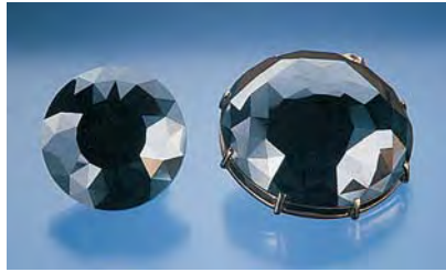
Figure 5. These round brilliants (the unmounted one weighs 10.30 ct) were represented as synthetic black diamond, but they were identified as very dark bluish green synthetic moissanite.
