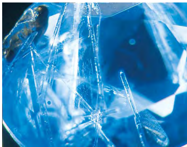
Figure 6. Elongate prismatic crystals, identified as apatite by Raman analysis, were seen in two of the h a y ne samples. Note also the piece of host rock evident on the surface of this sample, shown here at the upper left. Photomicrograph by H. A. H anni; magnified 30 .
