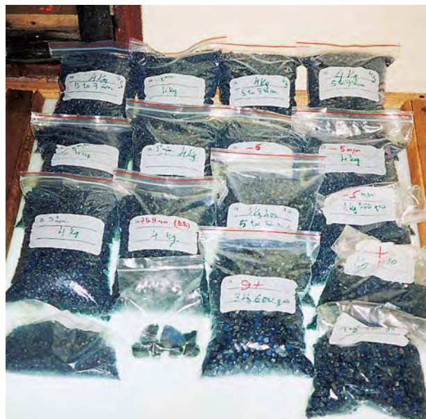
Figure 6. The rough sapphires are hand-sorted on light tables into separate quality and size categories. These parcels, totaling approximately 50 kg, were produced from the “M4” pit. Photo courtesy of Mega Gem s.a.r.l.
