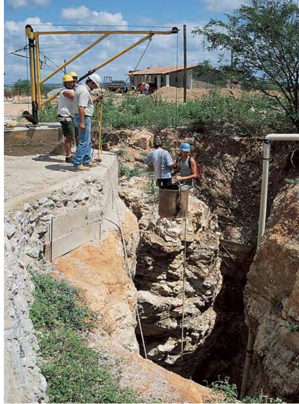
Figure 19. Gem-quality cuprian elbaite was reportedly recovered from this shaft at the Mulungu mine in Rio Grande do Norte State, Brazil. An electric winch and steel bucket are used to transport both miners and rock material. Photo by Brendan Laurs.
