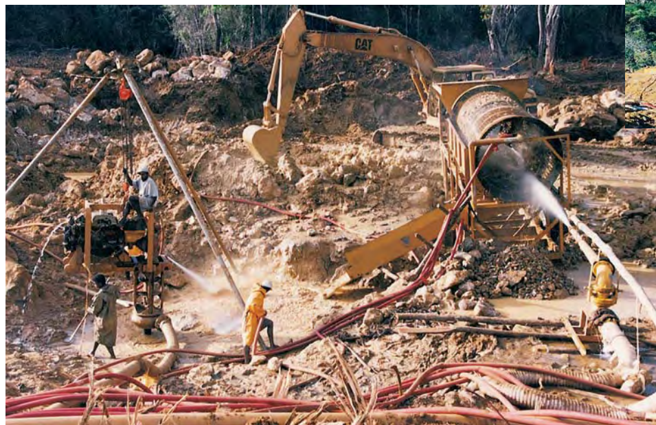
Figure 5. At this mechanized operation in the Anivorano area (the “M4” pit), a track-hoe dumps sapphire-bearing alluvium into a trommel (right). The gem-bearing gravel is then pumped from the small pit on the left to a nearby washing plant (see inset). Photos courtesy of Mega Gem s.a.r.l.
