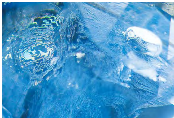
Figure 8. Commonly seen in the haüynes examined were well-formed negative crystals with rosette-like healing fissures (right, within the bright spot) or partially healed fissures with interference colors and a worm-like "fingerprint" structure (on the left). Photomicrograph by H. A. Hänni; magnified 40×.
