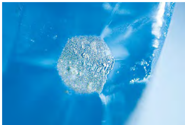
Figure 7. This hexagonal opaque crystal exposed at the surface of a polished haüyne was not identifiable with Raman analysis, possibly because it was metallic or too decomposed. Photomicrograph by H. A. Hänni; magnified 50×.
