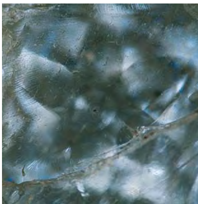
Figure 3. The gray "flower" in this 6.23 ct rough diamond (left, magnified 20 \times ) is caused by concentrations of hydrogen. Concentrations of pinpoints produce a "star" shape in the 0.71 ct Fancy Deep brownish orange round brilliant on the right. In both cases, the morphology of the growing diamond crystal controlled the shape of the inclusions.
