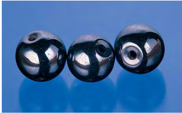
Figure 21. Represented as hematite, these strongly magnetic beads proved to be manufactured barium iron oxide. The beads measure approximately 8 mm in diameter; photo by Maha Tannous.
