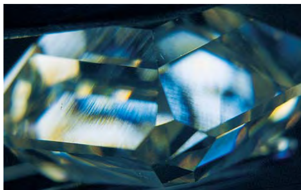
Figure 5. As is typical for type IIa diamonds, all of the samples studied showed tatami and banded extinction patterns with first-order interference colors when viewed between crossed polarizers. Photomicrograph by Christopher P. Smith; magnified 14 \times .
