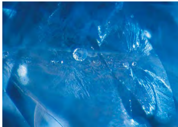
Figure 9. This rounded negative crystal has a frosted surface and, like the smaller negative crystal on the lower right, a rosette-like healing fissure. Photomicrograph by H. A. Hänni; magnified 40×.
