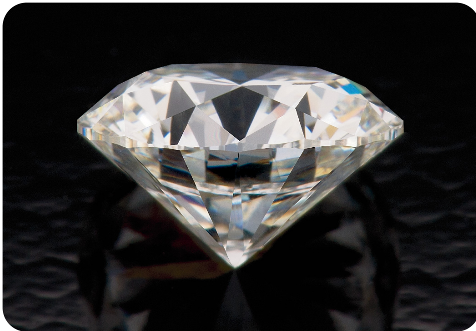
Figure 1. This 0.69 ct standard round brilliant cut diamond displays several obvious symmetry features that can be quantified. Photo by Robert Weldon.
