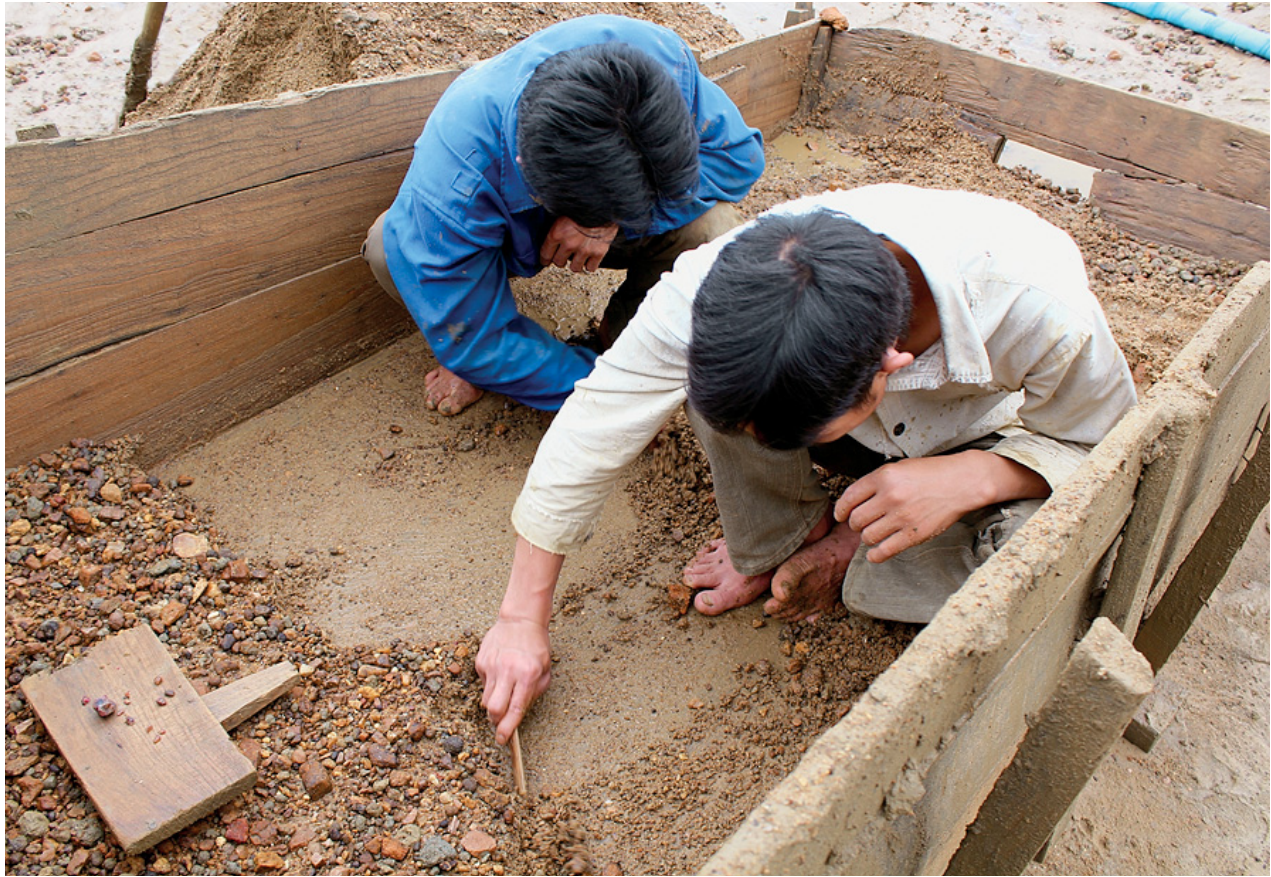
Figure 24. The spinel-bearing soil from Khuoi Ngan is washed and carefully sorted by hand to extract the small pieces of spinel. Photo by Dudley Blauwet.
