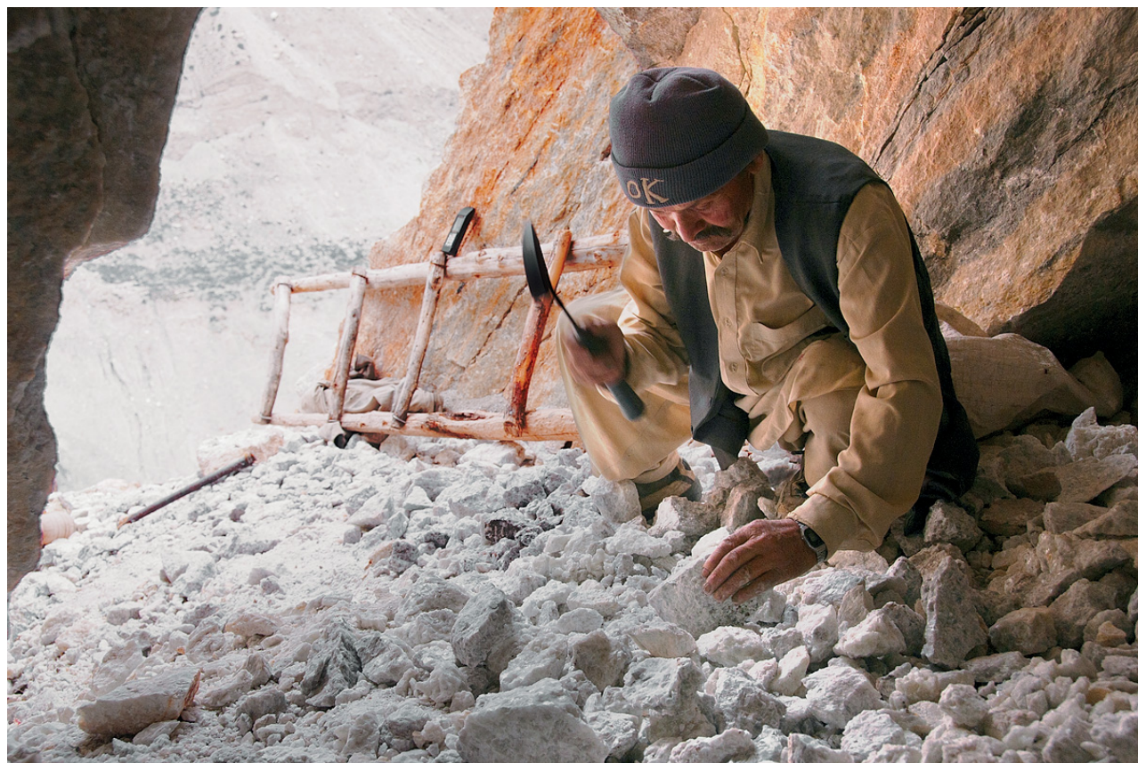
Figure 17. A Pakistani miner breaks marble to collect rubies at Datumbaresho, in the Hunza Valley. Photo by V. Pardieu.
