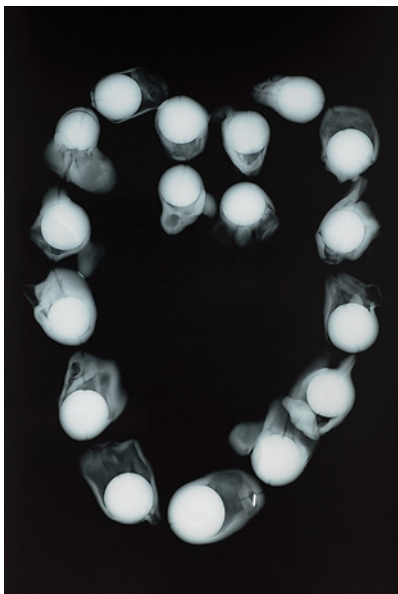
Figure 17. X-radiography of the strand reveals a bead-cultured structure and very thin nacre layers around the beads.
