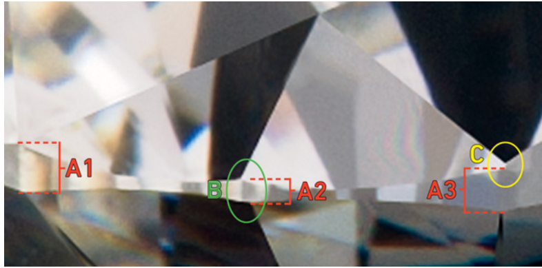
Figure 3. Three vertical lengths (A1–A3) in this close-up of the 0.69 ct diamond in figure 1 illustrate girdle thickness differences. Region B (green circle) shows where the facet edges of the upper and lower girdle do not meet (crown and pavilion misalignment). Region C (yellow circle) shows the junction where three facets fail to meet (pointing fault). Photo by Robert Weldon.
