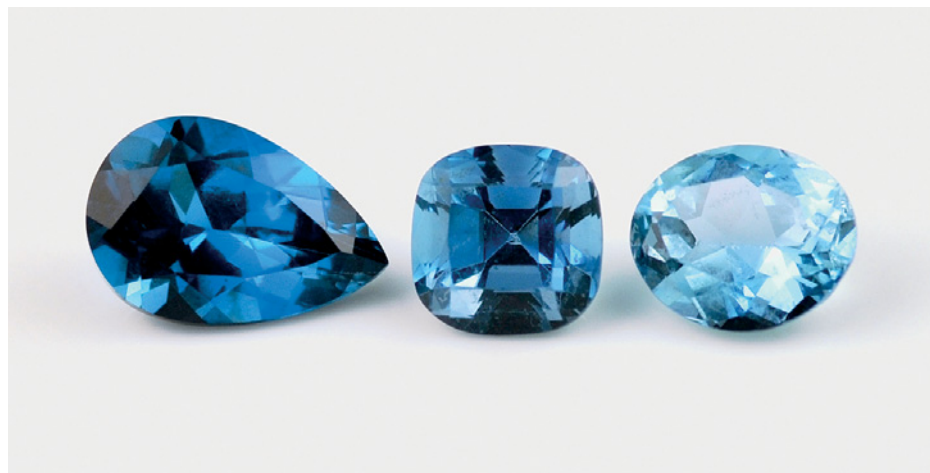
Figure 1. Most blue topaz on the market is irradiated to enhance its color. These stones (~4–10 ct) were treated by neutron irradiation. Photo by J. Zhang.
