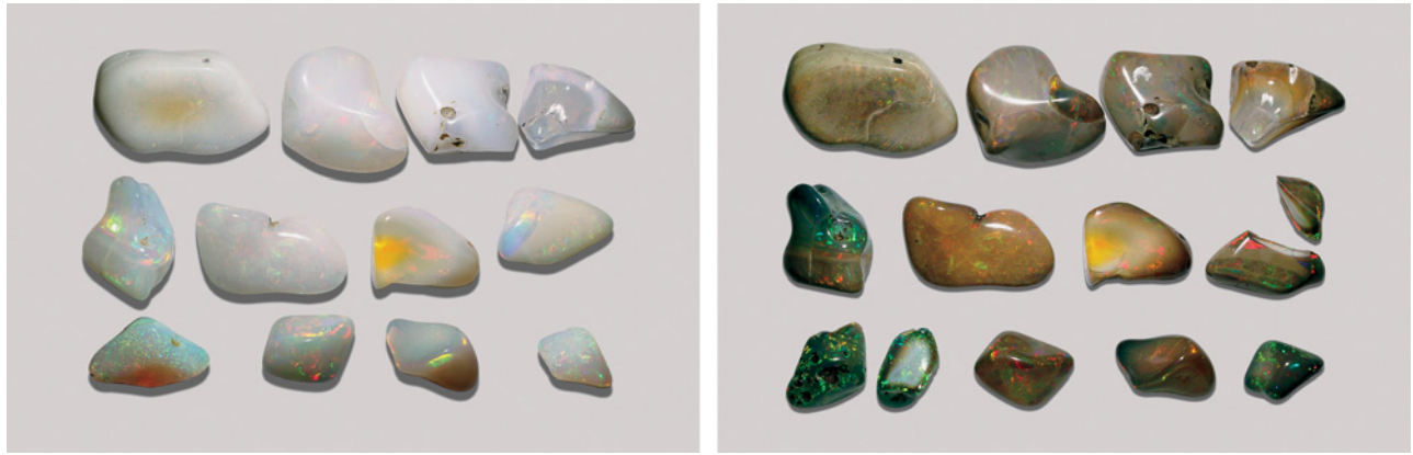
Figure 34. These opals from Wollo, Ethiopia, are shown before (left) and after (right) sugar-acid treatment. Darker bodycolors were produced in samples with a greater hydrophane character. The broken opals (center-right and bottom-left) show the shallow penetration depth of the treatment. The samples measure from 13 × 9 × 7 mm (lower right) to 29 × 16 × 10 mm (upper left). Photos by F. Mazzero.
