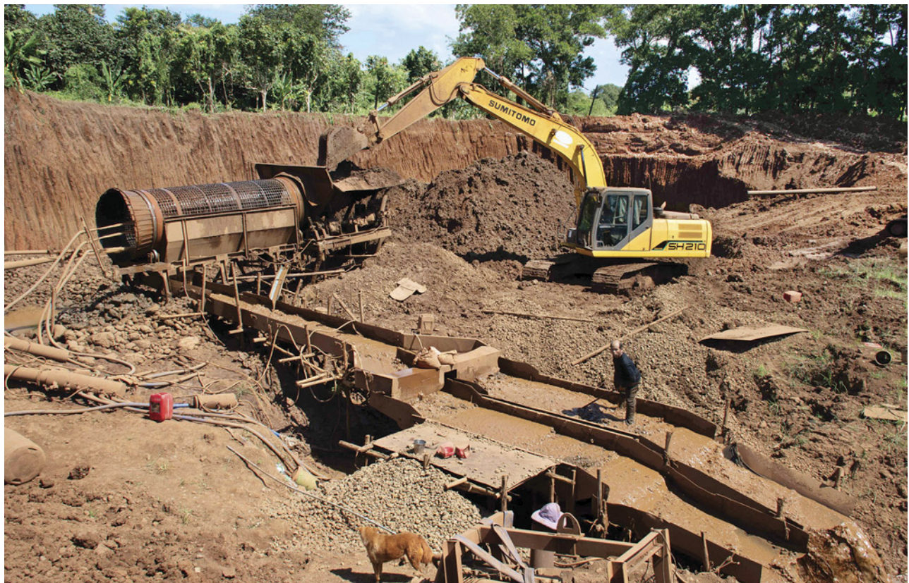
Figure 12. Mining of eluvial gem-bearing sediments from very weathered lava flows with mechanical equipment including a mechanical excavator, a rotating trammel cage to separate large rock pieces from the sediments, and a long sluice box to wash the sediments. This photo was taken in November 2020 at Khao Ploy Waen, an eroded volcano where sapphire is mined near Chanthaburi in eastern Thailand. Photo by Wim Verriest.
