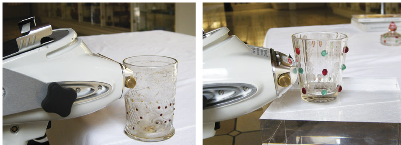
Figure 12. Examination of the beaker (left) and the lidded goblet (right) in the exhibition rooms of the Passau Glass Museum using a portable X-ray fluorescence analyzer. Photos by K. Schmetzer.
