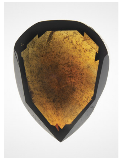
Figure 4. This 1.03 ct natural Fancy Dark brown diamond has uneven color zoning and abundant black inclusions. Infrared absorptions corresponding to carbon dioxide (2370 and 659 \text{cm}^{-1} ) and carbonate (1433 and 870 \text{cm}^{-1} ) were detected.
