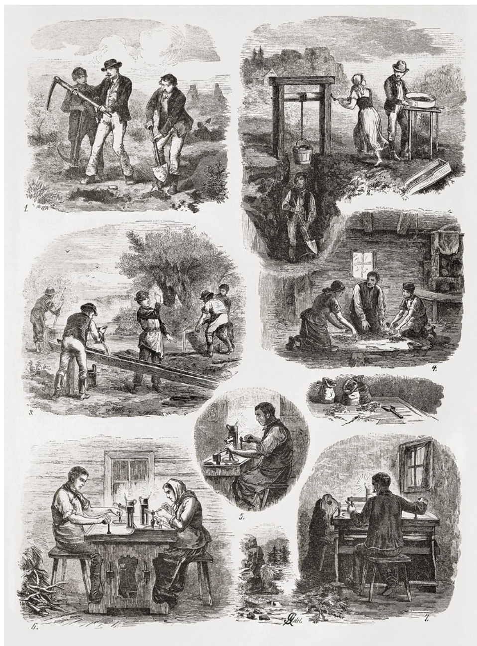
Figure 3. Extraction and processing of Bohemian garnets in the nineteenth century: (1) digging at the surface, (2) retrieving garnet-bearing soil or gravel from deeper levels and sieving, (3) washing to remove soil, (4) sorting, (5) cutting, (6) polishing, and (7) a view of the cutting table. From Gareis (1884).
