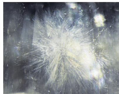
Figure 30. A fibrous snowflake-like inclusion found within the semitransparent thomsonite. Field of view 3.57 mm.
