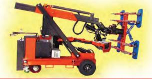
**The GM2000-12** This unit will lift a 2000 pound payload 13 feet into the air and place it using the best articulation in the business. This is the standard by which we compare the others.
