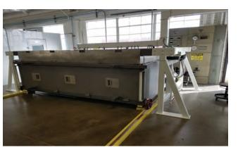
Bending Furnace for Ballistic Aircraft Glass
