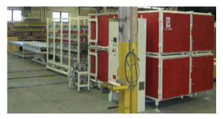
Vacuum Batch Laminating Systems Up to 1700 SF per 8 hour shift
