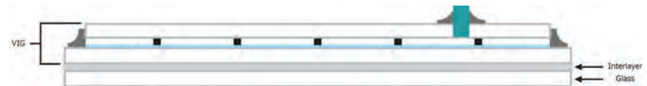
Diagram of a typical laminated VIG unit—a standard VIG unit bonded with an interlayer to an additional glass lite.
