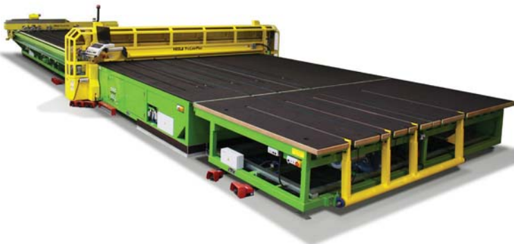
ProLam Plus Shape: Model cutting system for laminated glass
