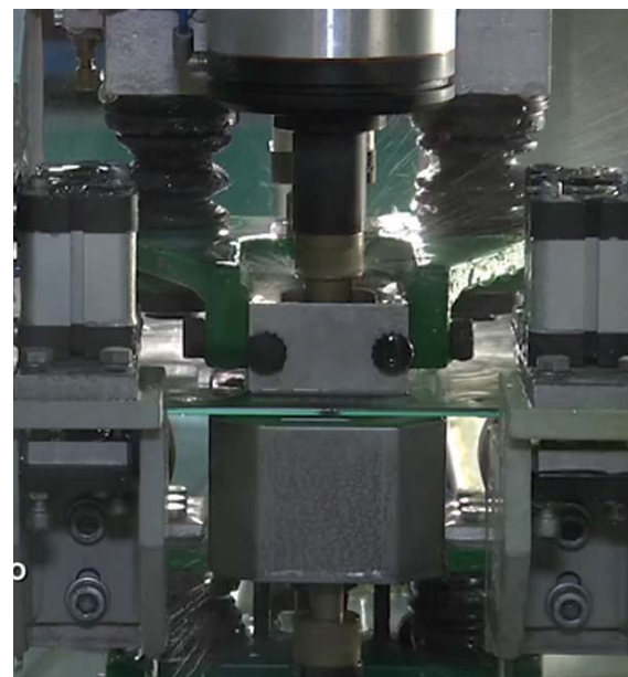
Vertical and horizontal drills: with facing heads, ranging from semi-automatic to CNC controlled versions and milling spindles, which can be equipped with tool storage and adapted as per the type of work to be carried out
