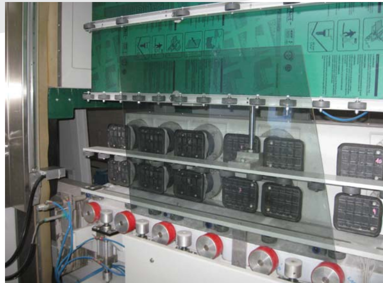
Vertical CNC grinder: it is a machine for grinding flat glass plates, both straight and shaped, which cup pick-up system, allows the processing of glass including low-E
