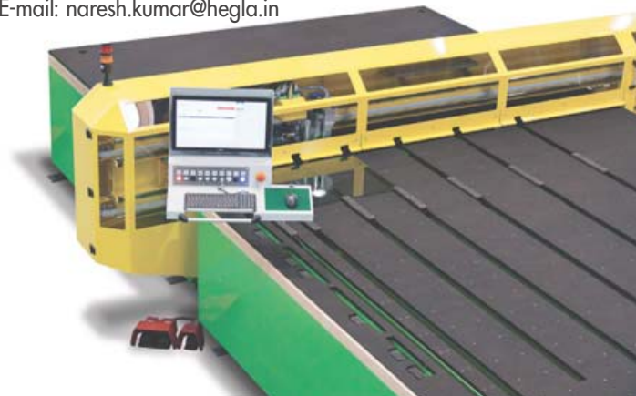
RapidLam: Compact model cutting system for laminated glass
