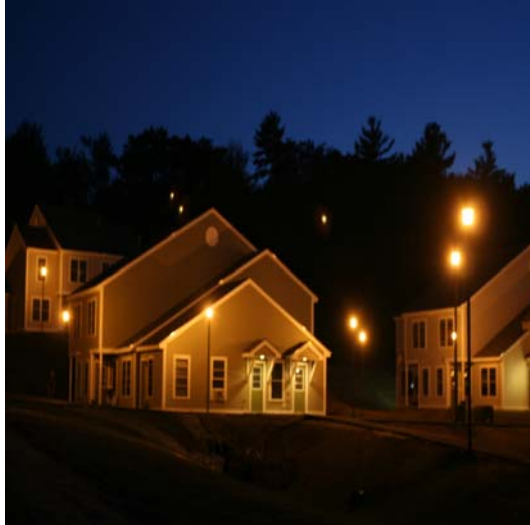
Intense, poorly shielded lighting illuminates rooftops, wasting energy and causing sky-glow
