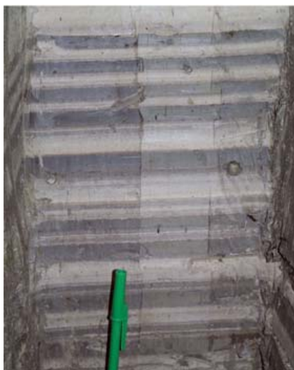
Chapter IV Figure 7. Varved clay. This glacial lake sediment consists of alternating layers of clay and silty sand. Each clay-silty sand couplet represents one year of sediment accumulation in the lake.
