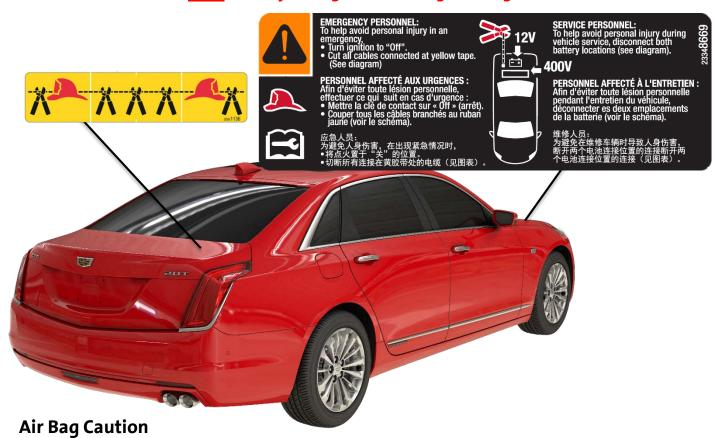
After disabling 12 volt power, wait at least 10 seconds to allow any un-deployed airbag reserve energy to dissipate.
