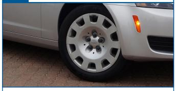
Plastic wheel cover attaches to threaded lug nuts
