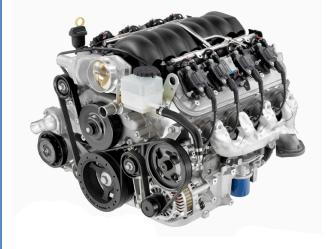
Replaces standard V6 engine with 6.0 liter V8. Sequential fuel injection with active fuel management cylinder deactivation. SAE Certified 355 horsepower @ 5300 rpm, 384 lb-ft torque @ 4400 rpm. Aluminum block with six-bolt, cross-bolted main-bearing caps, and aluminum heads with overhead valves.
