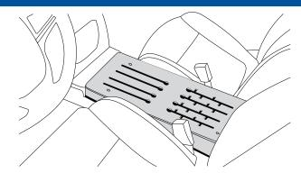
Center front equipment mounting platform between front seats, 27x9 inches, slotted for T-bolt attachment of customer equipment.
