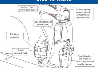
An auxiliary power junction block is located at the right side of the trunk. The junction block is at the rear of the auxiliary battery tray and contains a split buss with two terminals for customer connection to 12-volt battery power.
