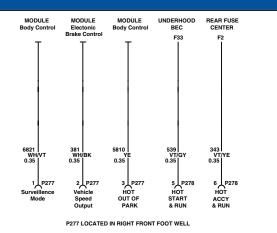
Ignition controlled power and signal circuits are also included in the 6 cavity and 16 cavity upfit connectors.
