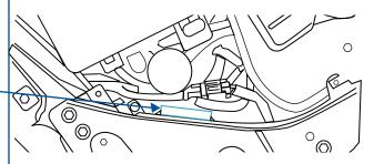
Option 6J7 provides a headlamps high beam flashing module, rear lamps flashing via the Body Control Module (BCM) and a control wire for customer-furnished switching to turn the module on and off. The flasher control wire is terminated in the 16-way connector on the upfitter harness at the right front corner of the equipment mounting platform. The flashing module is located is located on the rear side of the passenger side upper radiator support
