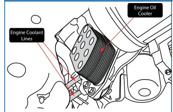
The oil-to-coolant engine oil cooler system is mounted on the left side of the lower engine block, forward of the oil filter. Engine oil flows through the stacked plate cooler from the engine oil sump and returns to the engine. Coolant flows to the cooler via a short hose from the engine block and exits to the radiator through a coupled hose connection to the radiator inlet hose.
