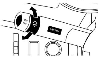
The DIC is operated via the controls on the Turn Signal lever at the left side of the steering column
