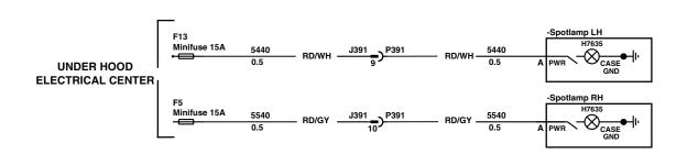
7X6 spotlamp left hand and 7X7, spotlamps left and right hand, pillar-mounted Unity, 6-inch with replaceable H3 halogen bulb; independently fused
