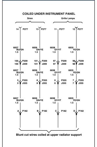
The SEO 6J3 wiring provision circuits are terminated in the 16 cavity connector at the front of the equipment mounting platform on the passenger side. The wiring circuits are routed from the passenger compartment to a 2 foot (30 cm) coil secured in the area behind the grille. There are four 16 gauge (1.5 mm) wires for connecting to the grille lights and siren speaker.
