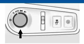
**WS** – Delete Daytime Running Lamps and Automatic Headlamps. This option disables the Daytime Running Lamps and Automatic Headlamps control feature. Exterior lamps are manually controlled only. Option VVS is not available in Canada. The headlamp control on the driver's side of the instrument panel operates the headlamps.
