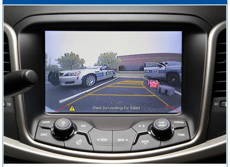
8-inch backup display with steering path guides displayed in radio screen.
