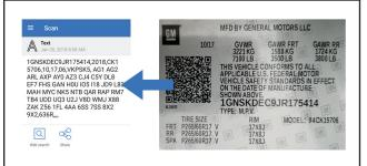
A Service Parts Identification (SPID) Label provides Vehicle Identification Number (VIN)-specific Option Code content list, Engineering Model Number (Nameplate, body style), Exterior paint system, Exterior paint color code and Interior trim level and color.
