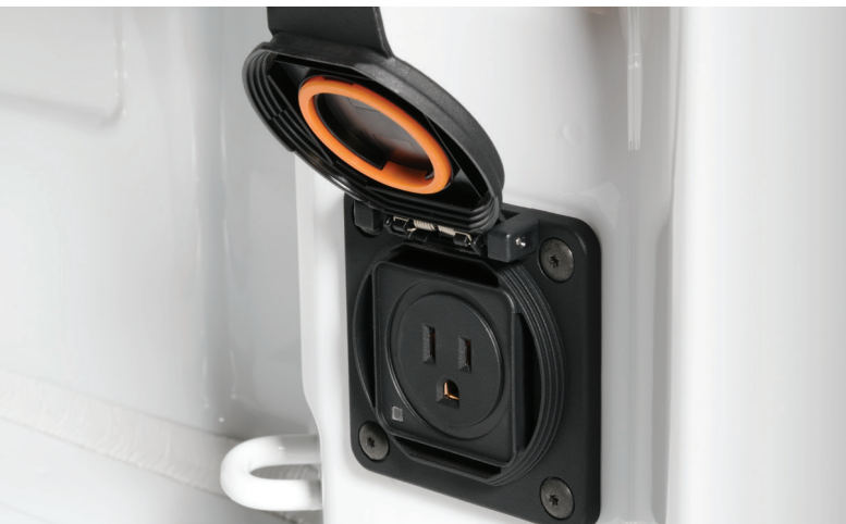
Standard 120-volt power outlet in bed
