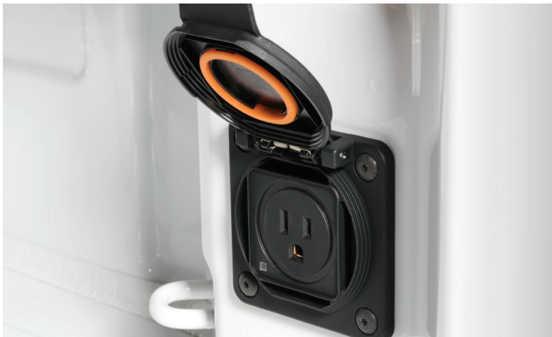
Standard 120-volt power outlet in bed
