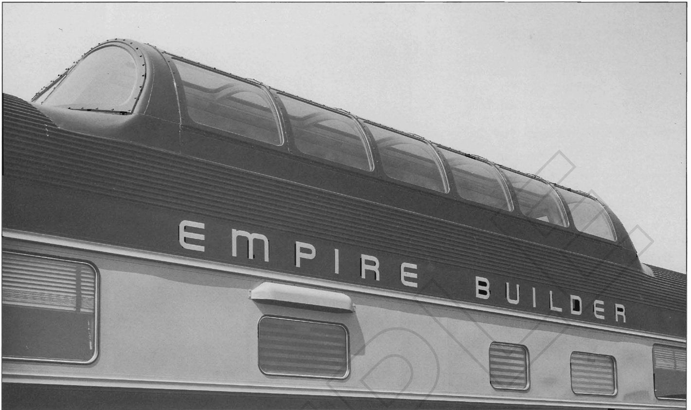
A close up of the construction of the coach dome, with its curved windows. The glass was tinted, and the GN took special pains to inform its passengers of the correct method of compensating exposure and color correction for good photographic results. A special brochure with technical discussions and correct filters and type of color film to use was available for all passengers.
