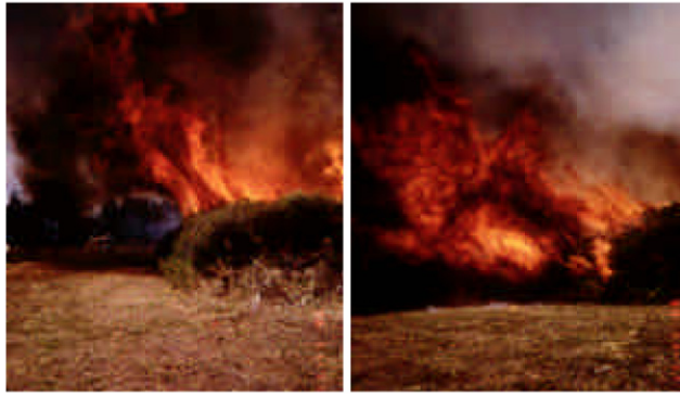
Figure 9 —Example of flame front collapse in New Zealand manuka shrub fuels during experimental burning trials observed from consecutive photographs.
