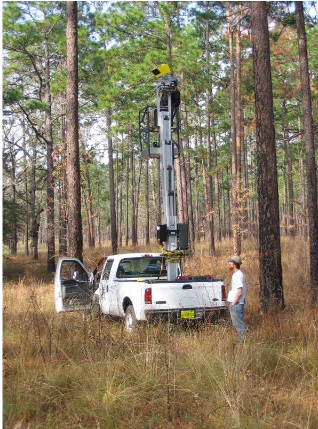
Figure 1 —A ground-based LIDAR system: The MTLs (Mobile Terrestrial Laser Scanner) is used to mobilize Optech's ILRIS 3 6 D (yellow instrument) for collecting high-resolution 3D point-cloud laser data.
