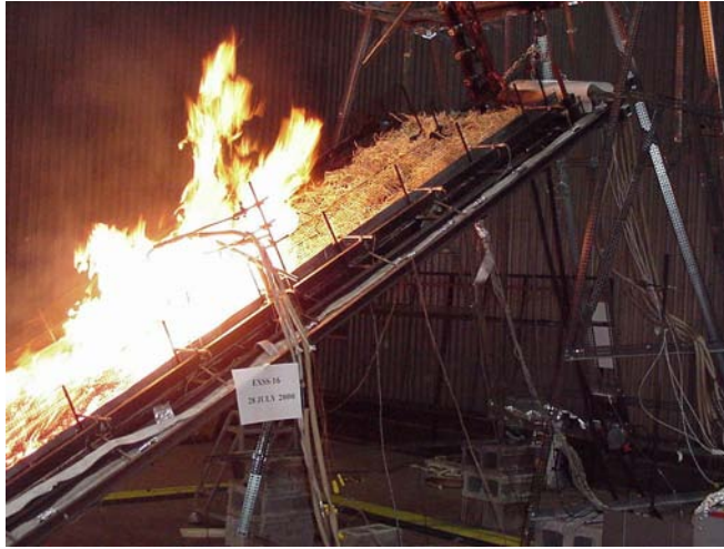
Figure 1 —Photograph of experiment, upward spreading fire, excelsior fuel, bed measured 1 m wide by 3.5 m long.
