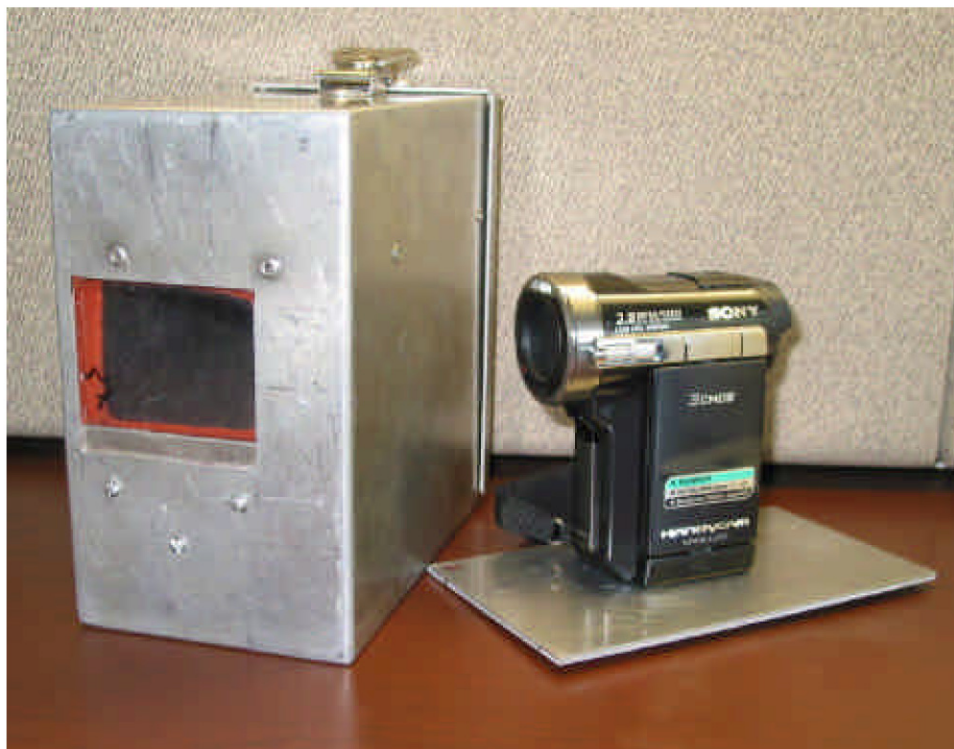
Figure 2—View of digital camera enclosure and camera mounting plate.
