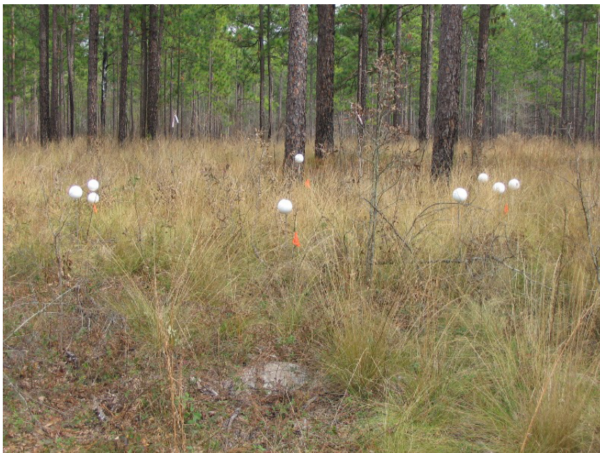
Figure 3 —Example of a 4 m x 4 m plot, with reference targets set up for ground-LIDAR acquisition and subsequent data processing.
