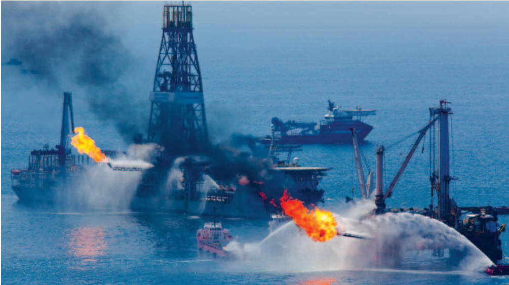
Transocean's huge drill ship the Discoverer Enterprise , its derrick towering 400 feet above the sea, and Helix's Q4000 (foreground) sit over the gushing wellhead. Together the vessels were able to recover up to 25,000 barrels of oil per day.
