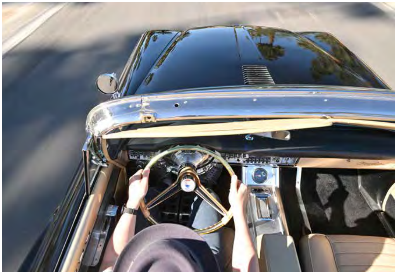
This 1960 300F is packed with contemporary technology, including push-button transmission controls and the AstraDome gauge package with electroluminescent lighting.
