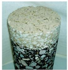
Figure 1: Light coloured asphalt
