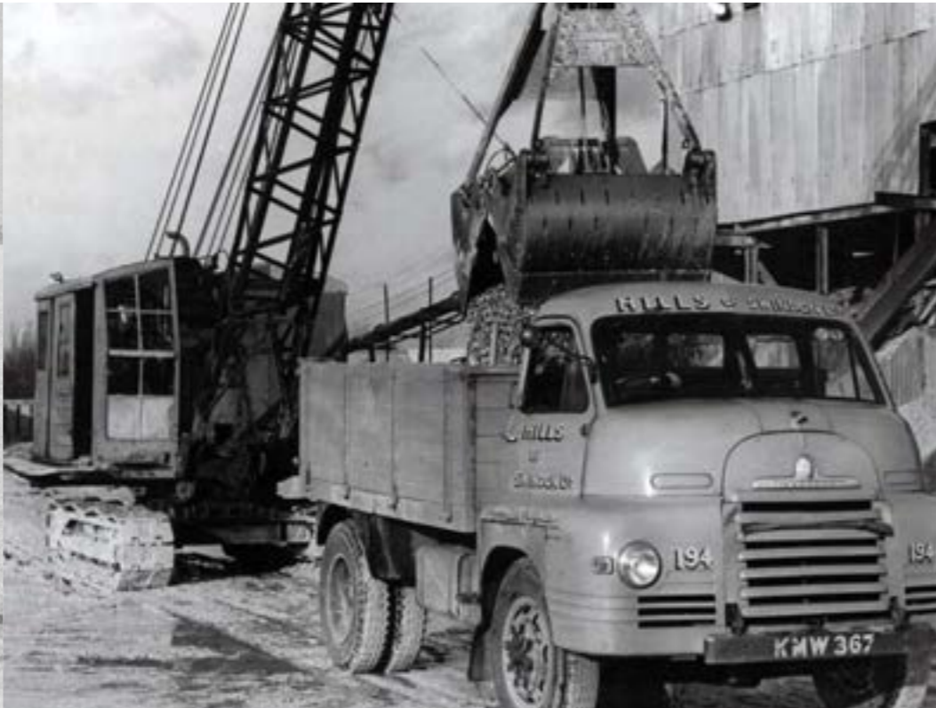
A Ruston Bucyrus excavator with grab loading an S-type petrol Bedford six-tonne tipper at the Broadway Lane North Gravel Plant, South Cerney.
