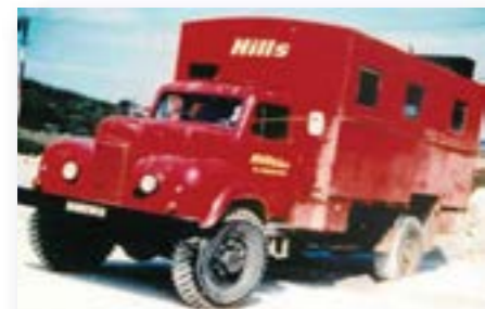
Commer Superpoise 4x4. The wonderfully named 'Superpoise' was formerly a military vehicle that Hills converted to a mobile workshop complete with welding equipment to support the plant hire business.
