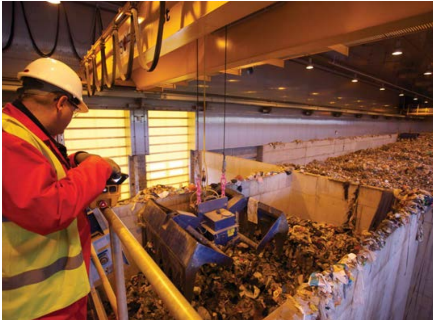
The main hall at the Northacre Resource Recovery Centre - transforming domestic waste into a fuel to generate electricity.
