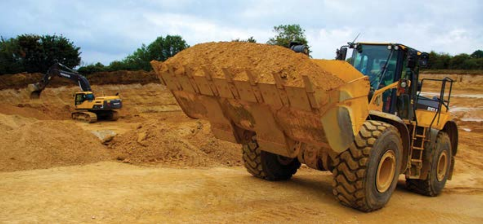
Mobile plant extracts sand from the Shorncliffe Quarry.
