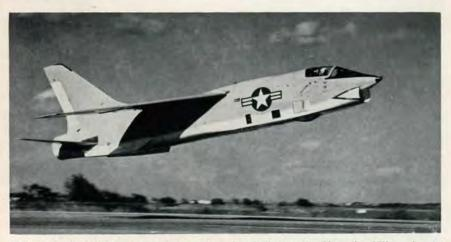
FIRST RF-8G PHOTO reconnaissance Crusader, built for the Navy by LTV, makes its maiden flight from Dallas, Texas on August 31. Originally designated the RF-8A, it has undergone structural changes along with the addition of ventral fins, wing pylon stations, and new camera positions. The first flight was made by Joe Engle, LTV test pilot. Fifty-three of the Navy's photo Crusaders are being modified to the new configuration.
