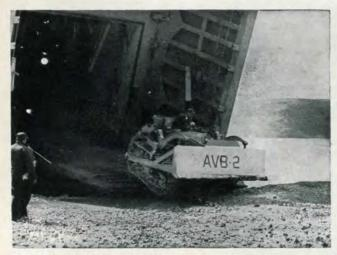
THE BULLDOZER is first off the ship. It is used to scrape a road to the ramp for the other vehicles and carves a runway, if needed.
