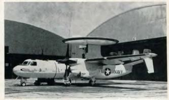
retrieve badly-needed repaired items. The E-2A Hawkeye (R) is shown with AN/APS-111 radar and AN/APA-164 rotodome installed. This new system provides improved definition of approaching aircraft and reduction of ground clutter. The Hawkeye will make its first appearance with the Seventh Fleet by the end of this calendar year.
