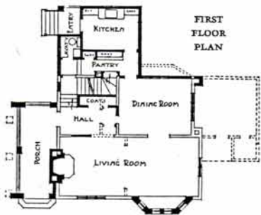
THE HOUSE BEFORE AND AFTER MOVING AND REMODELING. A NEW SERVICE WING WAS ADDED AND THE HOUSE WAS PLACED ON THE NEW LOT AT RIGHT ANGLES TO ITS OLD ORIENTATION. ROWE, DILLARD & ROWE, ARCHITECTS
