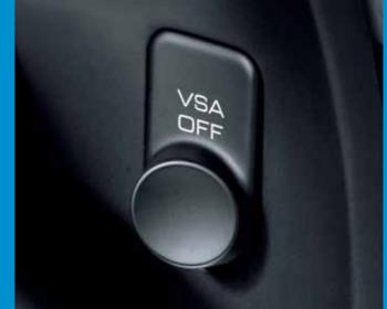
The Vehicle Stability Assist (VSA) system fitted as standar
