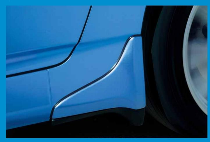
To provide the finishing touch to the Honda \$2000's smooth lines, fender lower protectors are available. These further smooth the airflow past the car's impressive rear tyres.
