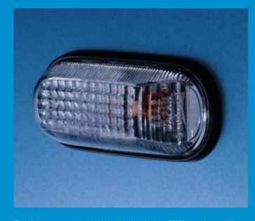
The indicator repeaters are located high on the side of the Honda S2000 for maximum visibility and
