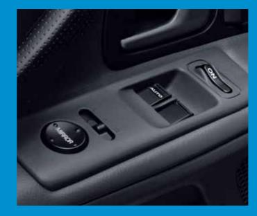
Electric window and remote mirror controls are all clustered together within the driver's doo. panel for ease of operation.
