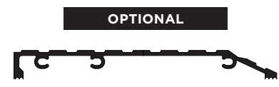
1/2" Tileback Aluminum Saddle Threshold (ADA) Tileback sill only available in 5" width. For use on a 4-9/16" jamb only.
