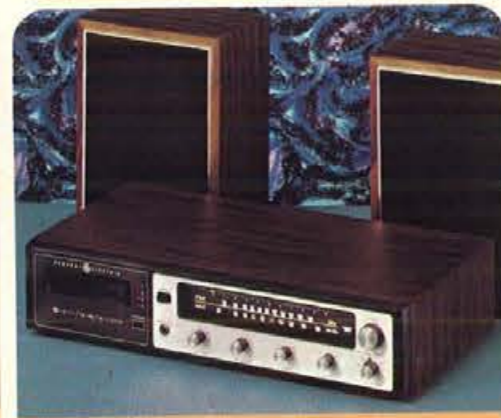
GE 8-TRACK STEREO TAPE PLAYER WITH FM/AM/FM STEREO TUNER. Plays 8-track stereo cartridges, FM/AM/FM stereo. 14 watts Peak Music Power (7 watts EIA Music Power). 6" high sensitivity speakers. "Stereo Star" and tape channel indicators. Jacks for Stereophone, Tape in/out. 19x4x10 \frac{1}{2} ". Enclosures: 9 \frac{7}{8} x7 \frac{1}{8} x5 \frac{1}{4} ". 25 \frac{1}{2} lbs. SC1080 S9475 ..... $129.95
