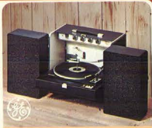
GE "TRIMLINE 500" AUTOMATIC STEREO PHONO. 14 watts Peak Music Power (7 watts EIA Music Power). Two 8" speakers. Stereophone jack, speaker on-off switch. Suspended 4-speed changer has ceramic cartridge with diamond stylus. Vinyl-covered steel cabinet. 24 \frac{1}{2} x9x14". Uses D5500 stand. 38 lbs. T541 S6750 Black ..... $99.95
