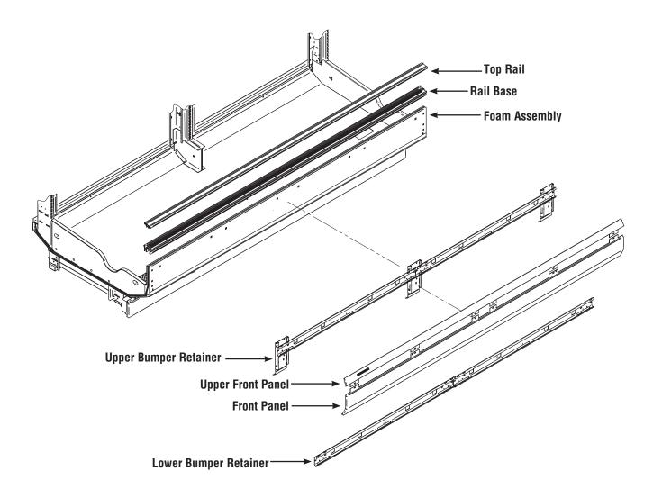
6. Verify that each merchandiser's upper front panel, front panel, and top rail align before joining merchandisers. Panels and top rail must have equal overhang at each end of the merchandiser.
