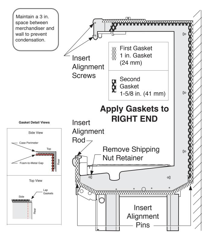
Gasket Location for Joining (Multi-deck)
