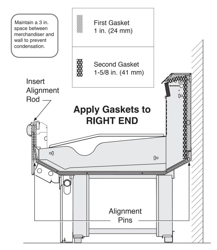
**Gasket Location for Joining (Single Deck)**
