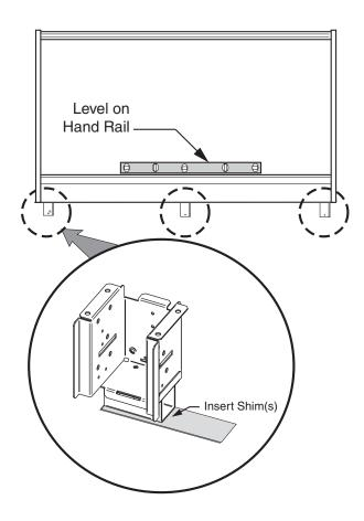
The merchandiser should be solidly supported at least every 4 feet (1220 mm). Once the merchandiser is level, if any gaps are present under the base rail, shims should be inserted approximately in line with the center front support legs to support the rear of the case. At the front of the case, insert shims under each of the center legs so that they support the front of the merchandiser.
