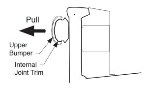
3. If not installed, install bumper end caps as shown below.
