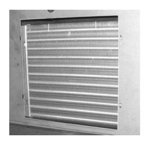
Airflow blockage increases energy consumption and reduces the merchandiser's ability to maintain operating temperature.
