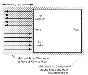
**GSVM-4072** (at 80°F/55% relative humidity, maximum ambient conditions) and **GSVM-5272** each require a 5 inch minimum clearance behind the merchandiser and clearance above the merchandiser since its air flows straight through the condensing unit compartment. Brackets are provided for field attachment to obtain this rear 5 inch minimum clearance.
