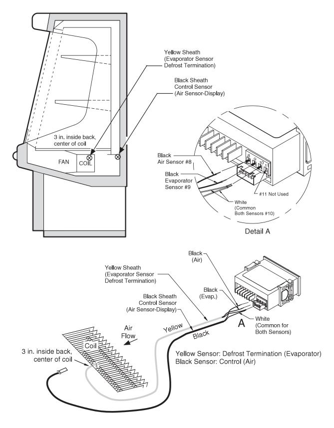
Typical Sensor to Control Configuration
