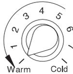
2. Rotate knob fully counterclockwise until it stops (full warm - "OFF" position)
