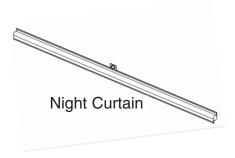
Carefully inspect the night curtain kit to ensure there is no damage from breakage during shipping. Case should be positioned and leveled before installing the night curtain.
