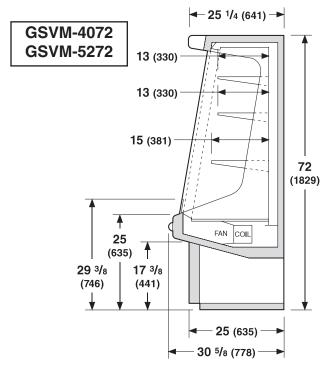
**Note:** This data is based on store temperature and humidity that does not exceed 75°F and 55% R.H. unless otherwise stated. Schedule defrost at night while lights are off.
