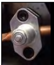
refrigeration line tapping valve
