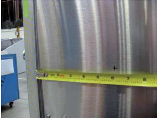
Step 1: Measure 6 inches from wrapping board end.
