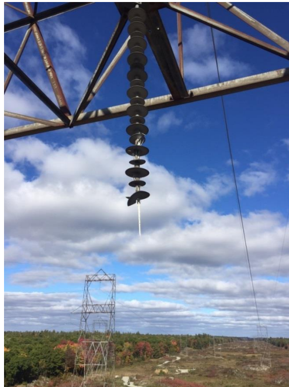
Figure 10: Failed Polymer Insulator
