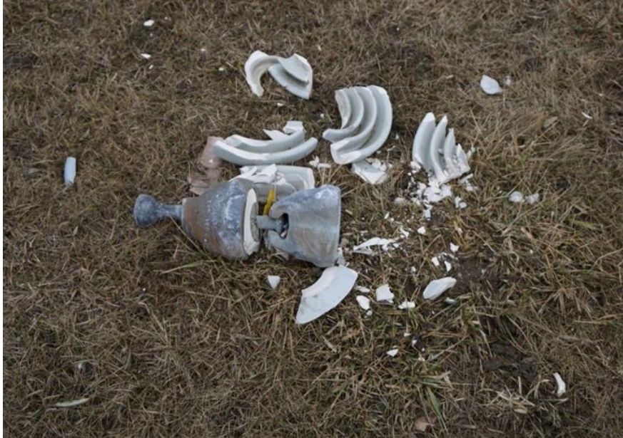
Figure 35: V76R Insulator Failure
