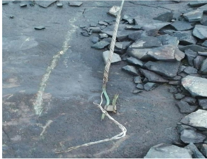
Figure 5: 2017 Shieldwire Failure on S22A
