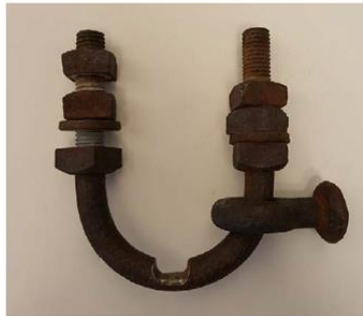
Figure 50: A Worn U-bolt
