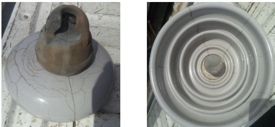
Figure 31: Porcelain Insulator Unit Affected by Cement Expansion
