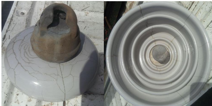
6 Figure 3: Porcelain Insulator Unit Affected by Cement Expansion
