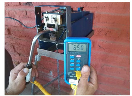
Pyrometer indicating proper blade temperature of 650°C.
