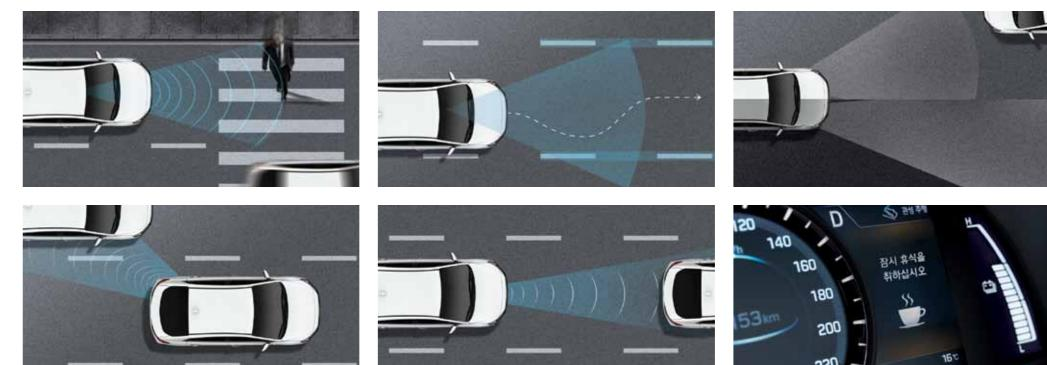
Front collision warning / Front collision avoidance assist Blind spot detection / Rear cross-traffic collision warning
