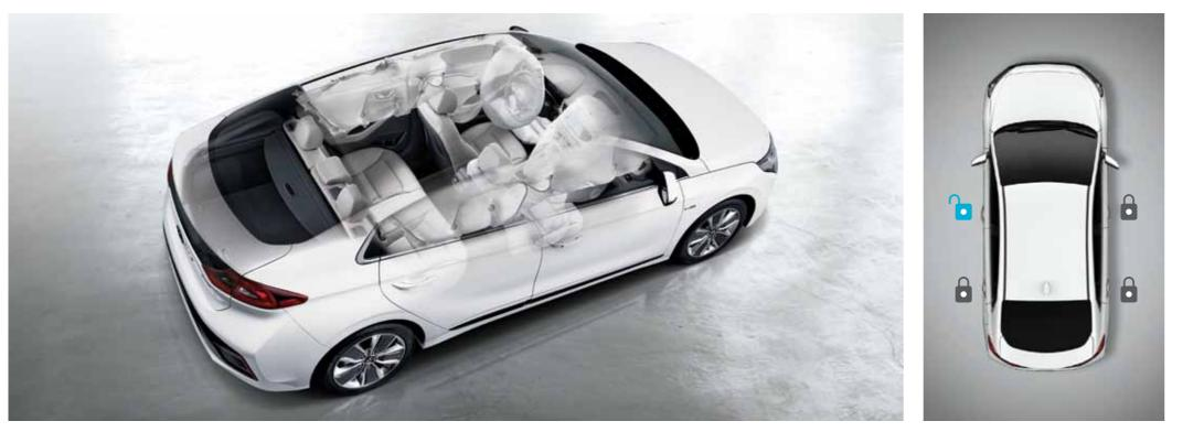
Seven-airbag system (advanced frontal airbags, driver's knee airbag, driver and front passenger side airbags, and curtain airbags)
