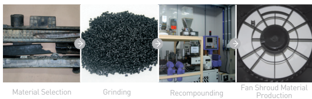
Recycling Process of Polyamide (Nylon) Parts
