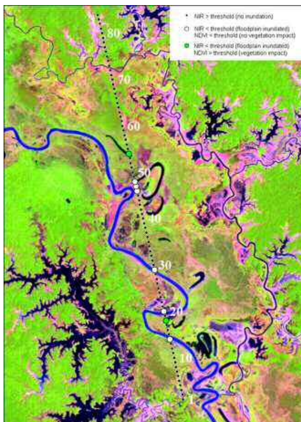
Figure 45. Landsat ETM7 (bands 5, 4, 3) on 28 th October 2002, waveforms located over inundated zones overlapping Envisat RA-2 18Hz waveforms pass 0677, cycle 10. White dots over water body are automatically selected (Marshall and Deng, 2016).
