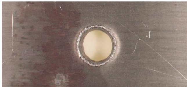
Figure 8. Front view of a perforated aluminum 0.5 inch thick target.
