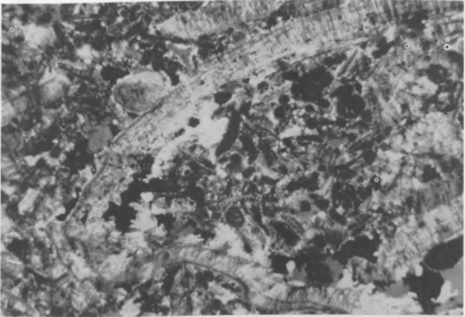
Fig. 2. An aspect of the texture of Hontoria limestone under the polarizing microscope. Differences in grain size are clearly observed.
