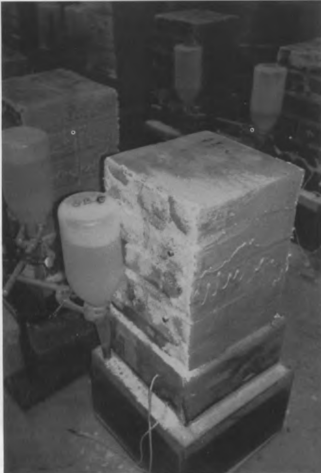
Fig. 6 Test walls for examination of rising damp. The piers are placed in a glass vessel with water.
