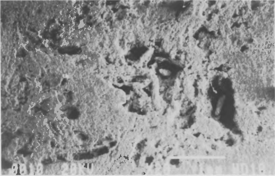
Fig. 4. Pores of different sizes in Hontoria limestone, observed with the scanning electron microscope (SEM).
