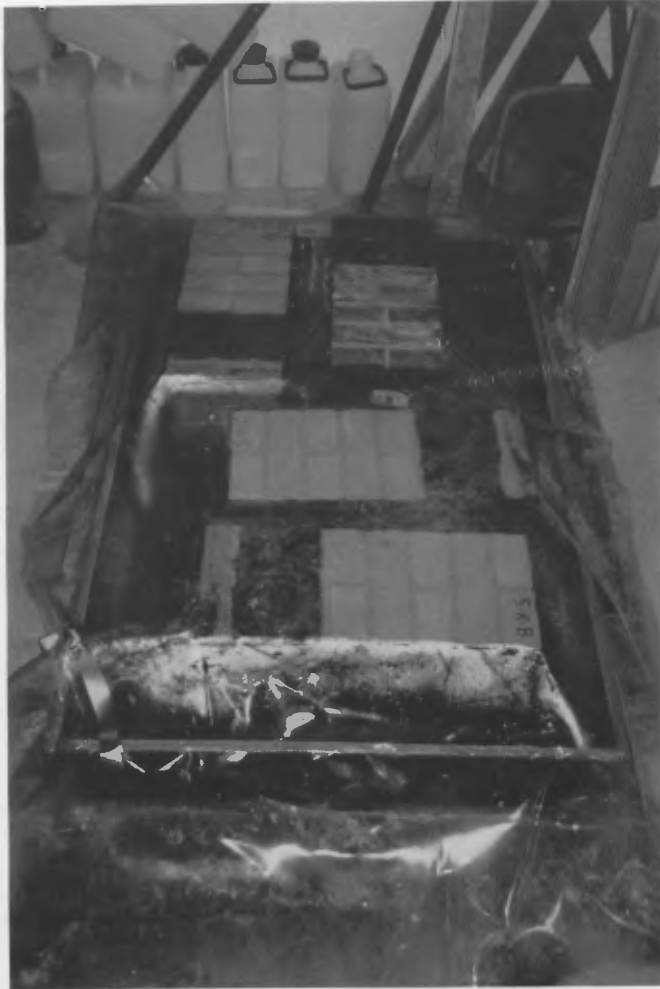
Fig. 5 Test walls for examination of rising damp. The piers are placed horizontally in a vessel with water (salt solution), for preliminary moistening. The vessel is covered with a plastic foil to prevent evaporation during this operation.
