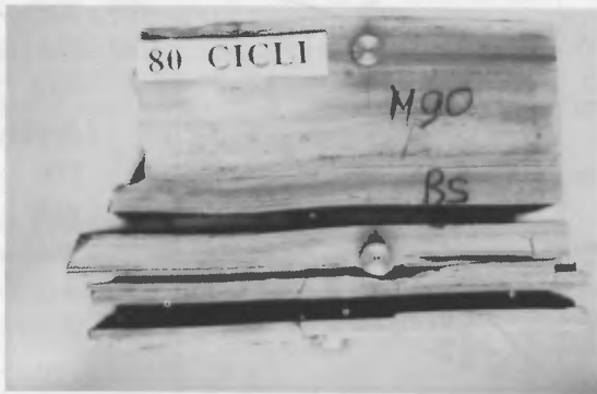
Fig.7. M 80 samples prior immersed for 3 days after freeze-thaw cycles indicated.
