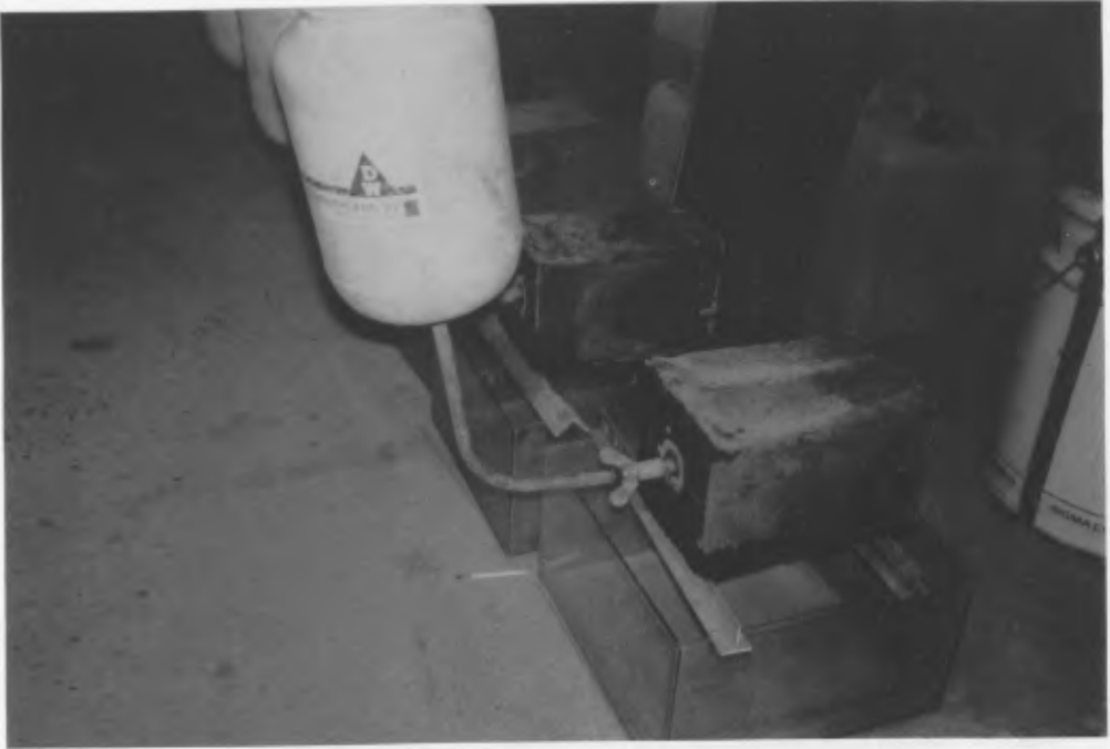
Fig. 2 Application under hydrostatic pressure (siliconate).
