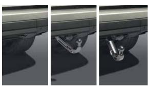
Electrically Deployable Tow Bar VPLGT0081, VPLGB0108, VPLGT0109, VPLGT0108
