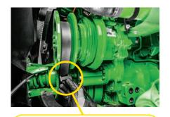
Checking Vari-Cool Fan drive belt width for wear is a very important routine maintenance step to avoid downtime. Use belt gauge R569237 shown in the picture above, which can also be purchased at your local John Deere dealer.
