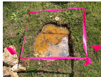
Soil percolation test
