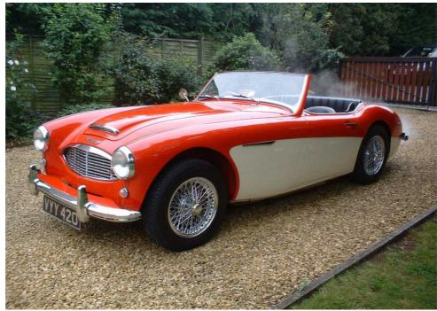
produce 120bhp. The suspension comprised 14-leaf rear springs and adjustable shock absorbers. Tony has replaced the rear suspension with standard kit (he says it made his eyeballs rattle!) but you can still see the evidence of the original front suspension in the gap between the tyre and the wing. The vehicle was
