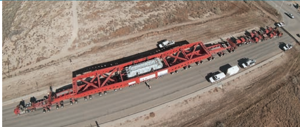
The gross weight of the heaviest load tipped the scales at 1.8 million pounds. At some locations, as many as nine trucks were attached to the load.
