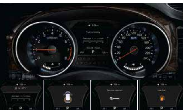
Supervision cluster (7" color TFT LCD) A high-visibility display located in the center gauge cluster provides useful, on-demand trip computer information graphics such as distance to empty, average and instant fuel consumption and outside temperature.
