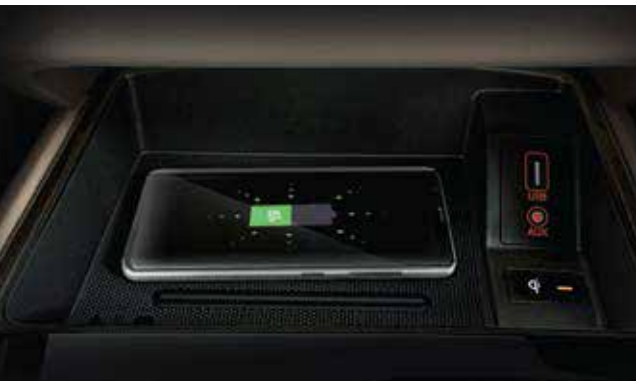
Wireless smartphone charger Charge a compatible mobile phone wirelessly on the pad at the front of the center console. An orange light indicates charging in progress; green indicates a full charge.
