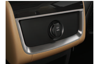
Center-console power outlet
