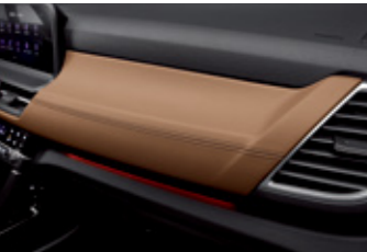
Crashpad in-mold stitching
