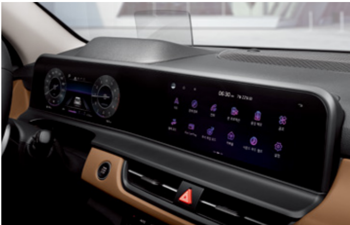
Panoramic display A panoramic display with an integrated 10.25" cluster and a 10.25" navigation system creates a simple, high-tech interior.
