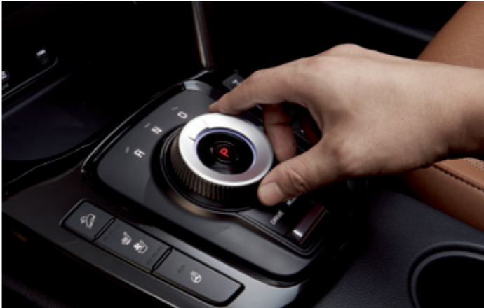
Dial type shift by wire system A sophisticated dial-type electronic transmission has a comfortable grip and delivers an elevated sense of luxury.
