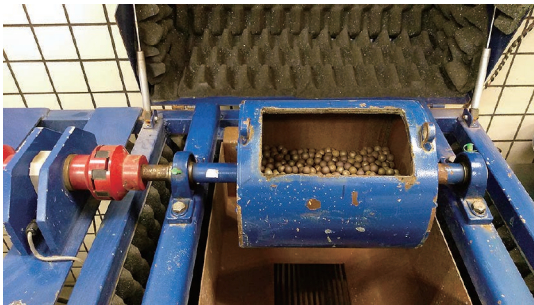
Fig. 1 8"×10" jar mill equipped with a torque sensor.
