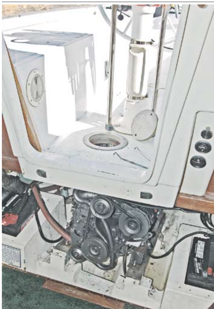
Diesel installations vary from boat to boat. On this one, you access the coolant reservoir and oil fill through a deck plate in the cockpit. Make sure you know how to access all the vital fluids on your motor, be it gas or diesel.
