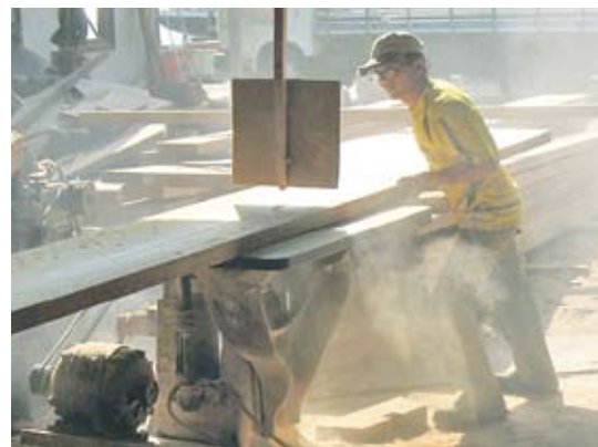
An Amazon shipwright shapes a new frame out of a massive plank of angelim vermelho.
